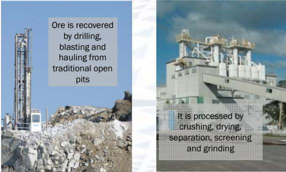
Ore is recovered by drilling, blasting and hauling from traditional open pits
