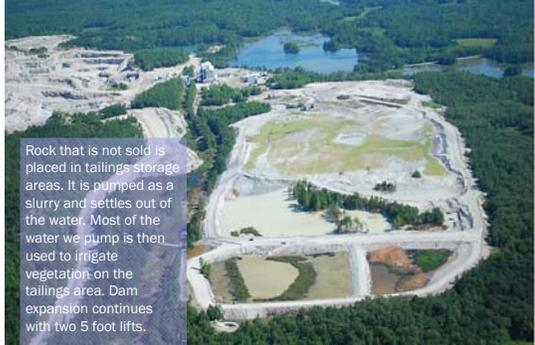
Rock that is not sold is placed in tailings storage areas. It is pumped as a slurry and settles out of the water. Most of the water we pump is then used to irrigate vegetation on the tailings area. Dam expansion continues with two 5 foot lifts.
